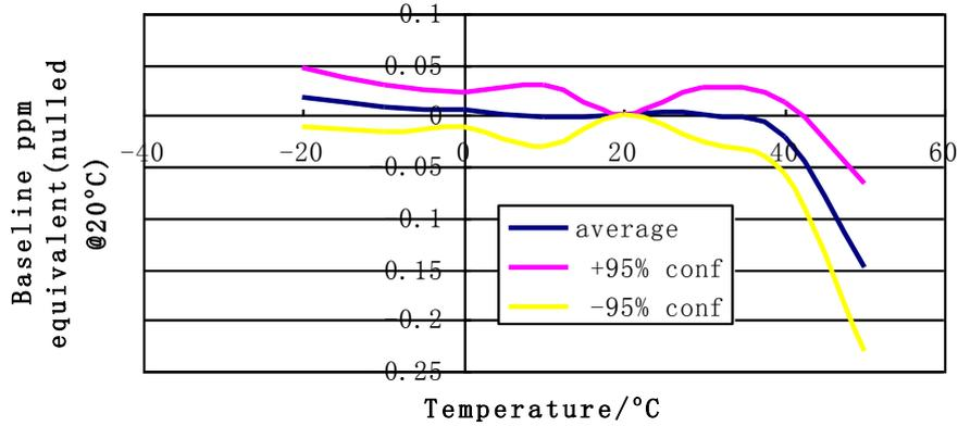
7R Cl<sub>2</sub> Sensor Sensitivity Temperature Dependence
